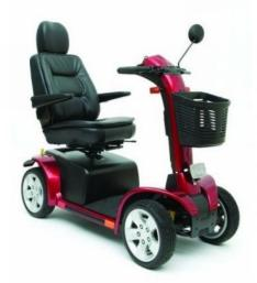
The Pathrider 130 XL mobility scooter features a powerful drivetrain and large 33cm (13") pneumatic wheels to handle rugged outdoor terrain. Luxury touches like a wraparound easy drive tiller, low-profile non-marking tyres, seat post suspension for a smoother ride and an LED curb light blend seamlessly giving the Pathrider 130XL a sleek, sporty style.
